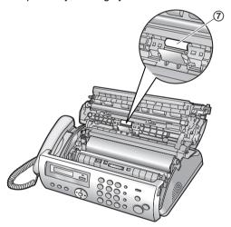
5 Close the back cover securely by pushing down on the dotted area at both ends (®), then close the front cover securely (③).
